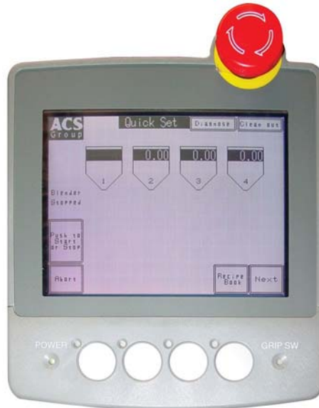
Figure 4: Typical Mitsubishi Controller Touch Screen Display
